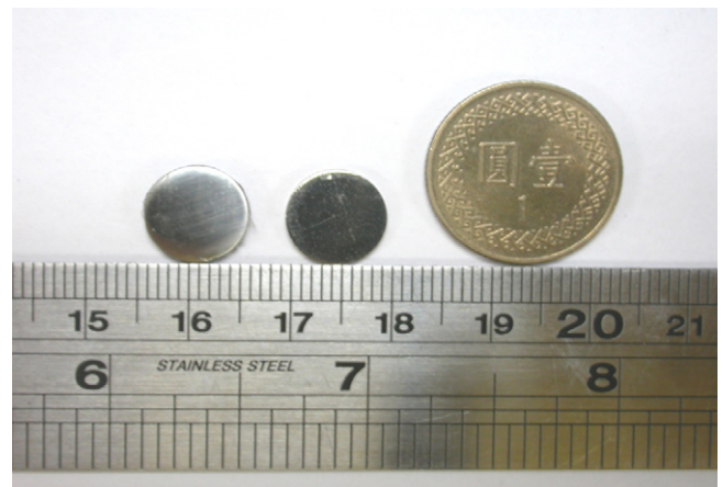
Fig. 3. The outer morphology of the Mg_{49}Y_{15}Cu_{36} BMG after vacuum hot pressing at 473 K with a pressure of 1.2 GPa.
